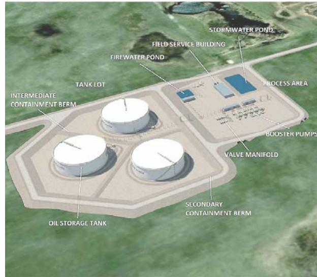
As part of its quarterly update on Energy East filed with the National Energy Board on Sept. 30, TransCanada released these updated proposed layouts of the pump station and tank farm to be added at the site of the Moosomin Compressor Station, which is located northeast of town. The tank terminal would include three 350,000 barrel tanks for a total capacity of 1,050,000 barrels of oil.
