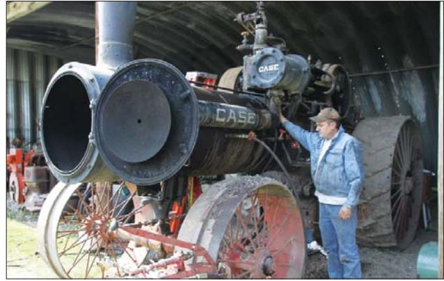
Hobbyist Robert Bryce stands beside the 1913-model steam engine that was repaired to working order at the Rocanville museum. Bryce oversaw the repair on the engine—a weld repair that was the first of its kind allowed in Saskatchewan.
