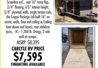
Screwless ext., rear 16" ramp flap, 3/4" flooring, 6'5" interior height, 3/8" plywood walls, single torsion axle, the Cougar Package (all built 16" on centre, walls, floor and ceiling w/ ceiling liner above roof bows), rear stabilizer jacks, (4) - 1,200 lb. Drings, 2 side wall air scoops.
