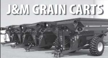
J&M grain carts use a single auger, which means there's no drag and less power requirements needed. Their front fold auger design gives you 100% visibility while unloading.
