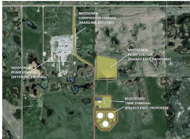
The proposed Energy East pipeline project would include a tank farm at the Moosomin compressor station and a feeder pipeline from Cromer to Moosomin.
