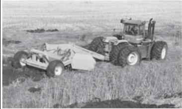
U-shaped blade gobbles up mountains of dirt. 18' model drags 15-18 cu. yds. 24' model drags 20 - 25 cu. yds. Six times faster than a scraper.
