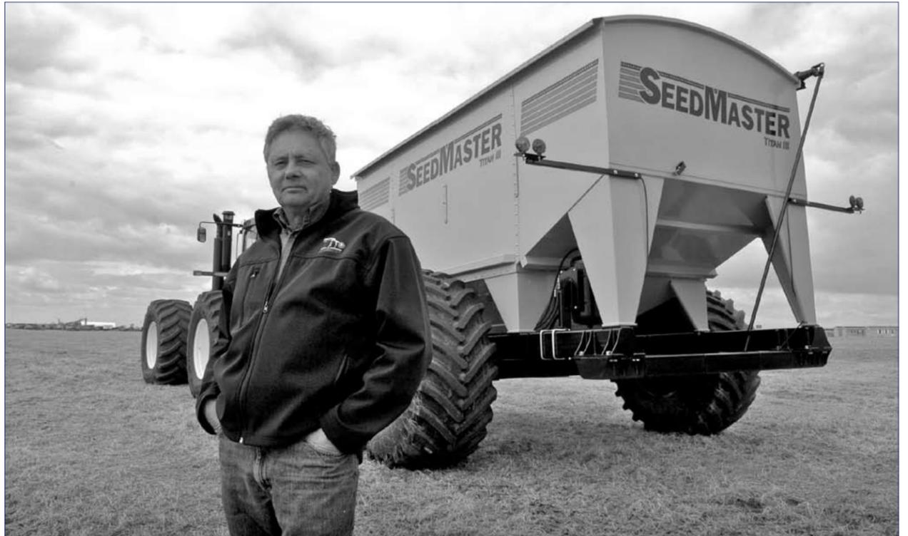
Norbert Beaujot, owner of the SeedMaster manufacturing plant near Regina, with the Titan III, a multi-use fertilizer tank that combines with SeedMaster's on-board seed tank to offer a 920-bushel carrying capacity—the largest of any commercial seeding tank system in North America.
