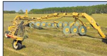
The VR683 Supersteer truly handles like a rake half its size. In field position, the VR683 pivot's around its center casters which cuts its wheelbase in half. The center casters are locked forward while the rear casters pivot freely. You'll have no problem making your headland turn in fields cut back and forth.
