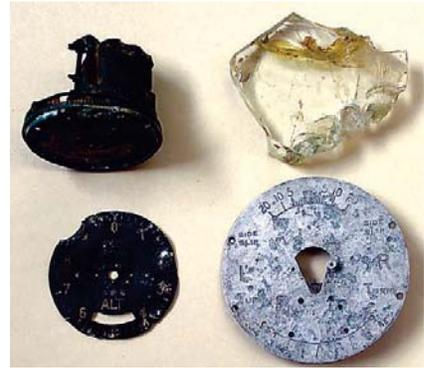
These pieces of Bev Smiley's downed Hurricane fighter were excavated in France. On the left are the guts and face plate of the altimeter. Top right is a piece of the Perspex or wind-screen, and at bottom right is the face plate of the Turn and Slip Indicator.
